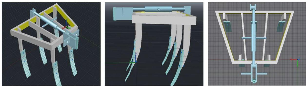
Figure 2 AutoCAD model of 5-tyne cultivator
