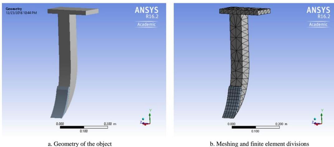
Figure 5 Cultivator tyne geometry
