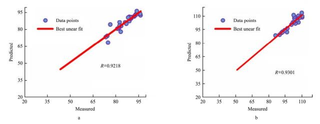
Figure 5 The ANN prediction for the cylinder head temperature (a) and cylinder block temperature (b) versus experimental values
