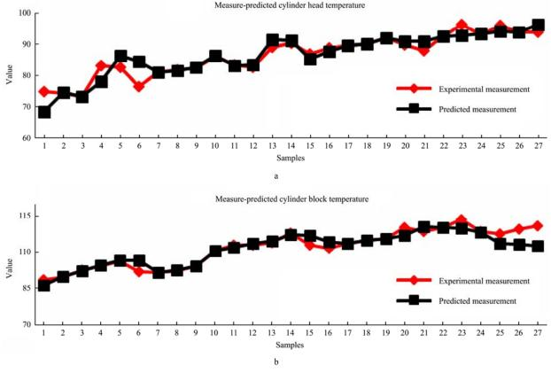
Figure 6 Comparisons of experimental results and the ANN predictions for the cylinder head temperature (a) and cylinder block temperature (b) for various test patterns
