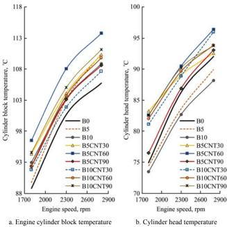
Figure 3 Diagram of engine block and head temperature at engine speeds of 1800, 2300 and 2800 rpm for different fuel blends
