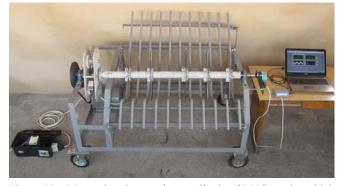
Figure 10 Measuring the angular amplitude of RVG carrier which is part of an experimental fruit detacher
