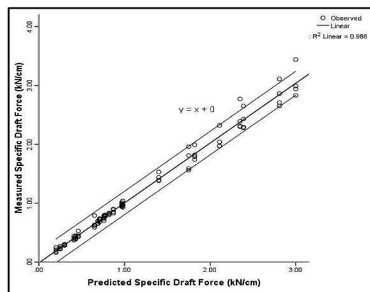
Figure 14 Line of fit between predicted and measured draft (Ndisya et al. 2016)
