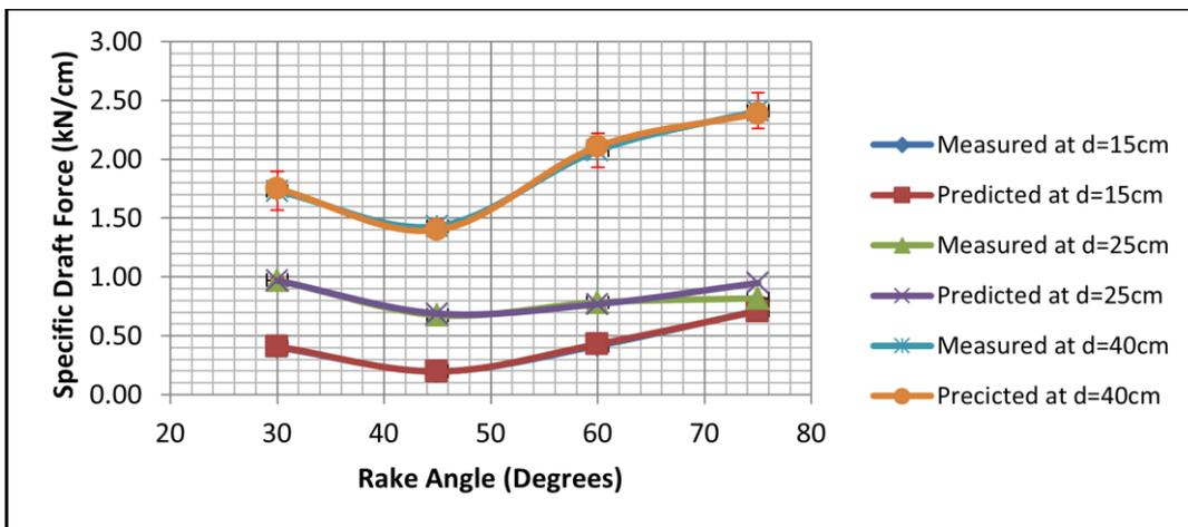
Figure 15 Specific draft against rake angle at operating speed of 3 kph
