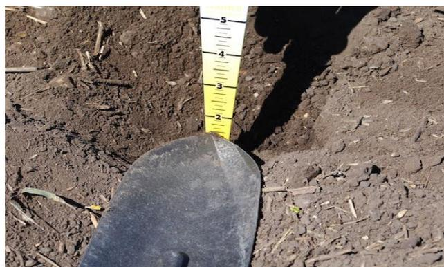
Figure 8 Furrow depth measurement (Canola Council of Canada 2016)
