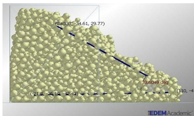
Figure 13 Slumped soil mass showing the angle of repose
