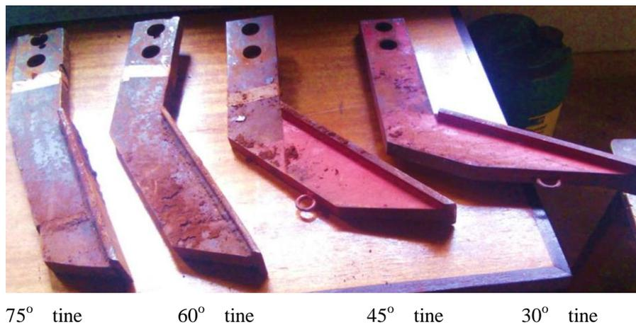
Figure 9 Ripper tines used (Ndisya et al. 2016)
