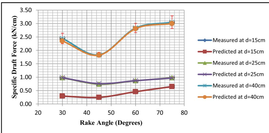
Figure 16 Specific draft against rake angle at operating speed of 5 kph
