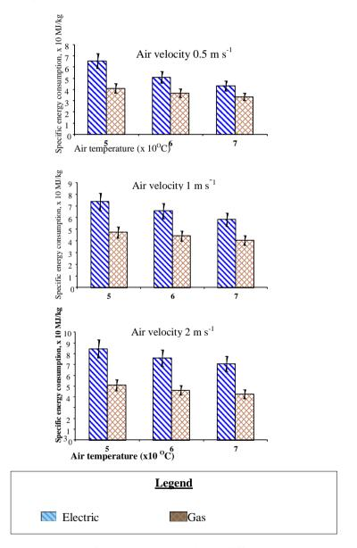
Figure 7 Specific energy consumption at different levels of drying air temperature and air velocity for both the electrical and the gas dryer as reported by El-Mesery and Mwithiga (2012)
