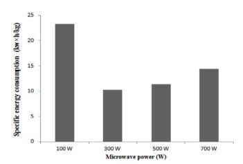
Figure 5 Specific energy consumption for microwave drying of carrot slices as reported by Zarein et al (2013).
