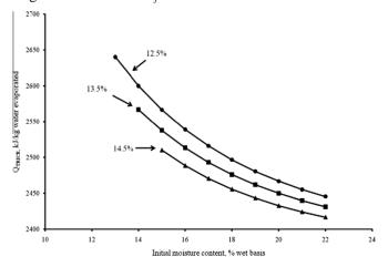
Figure 1 Total energy required to dry rice  $(Q_T)$  to 12.5%, 13.5%, and 14.5% (wb) moisture content of the long-grain, non-parboiled rice at 60 °C. (Billiris et al., 2011)
