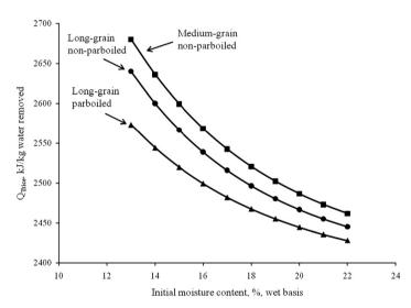
Figure 2 Energy required to dry rice  $(Q_{Trice})$  to 12.5% (wb) moisture content for long-grain non-parboiled, long-grain parboiled and medium-grain non-parboiled rice at 60 °C. (Billiris et al., 2011)
