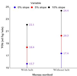
Figure 4 Effect of hip belt and shoulder strap supports (with and without) on oxygen consumption (VO<sub>2</sub>) at different upward slopes
