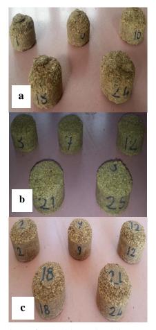
Figure 5 Views after tumbler testing briquettes produced at 115 MPa (a), 150 MPa (b) and 185 MPa (c) compaction pressure
