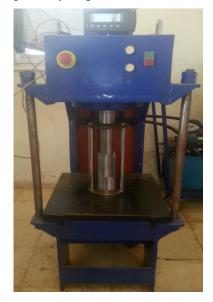
Figure 2 Hydraulic press and a punch-die set
