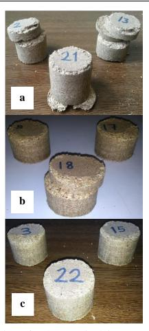
Figure 6 Views after shatter testing briquettes produced at 115 MPa (a), 150 MPa (b) and 185 MPa (c) compaction pressure
