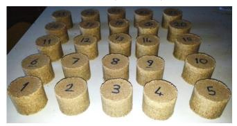
Figure 4 Samples of briquette obtained at 185 MPa
