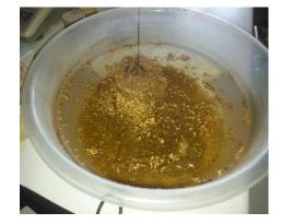
Figure 7 View of pepper crop briquette after water resistance test
