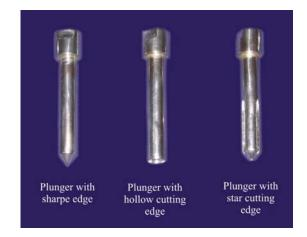
Figure 3 Pictorial representation of three types of plungers
