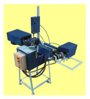
Figure 1 Continuous seed removing machine
