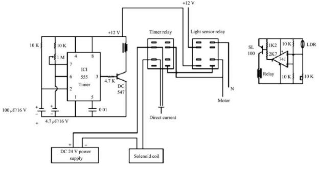
Figure 4 Circuit diagram of electronic control unit
