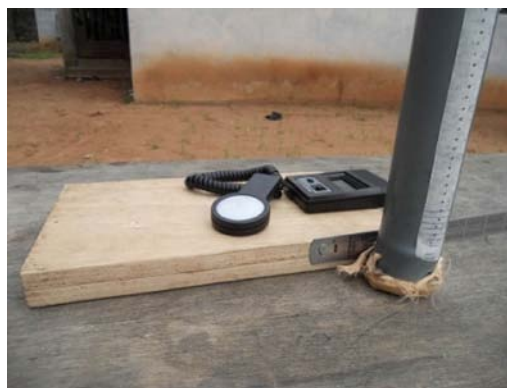
Figure 1 Flat plate surface solar collector with solar radiometer on horizontal position
